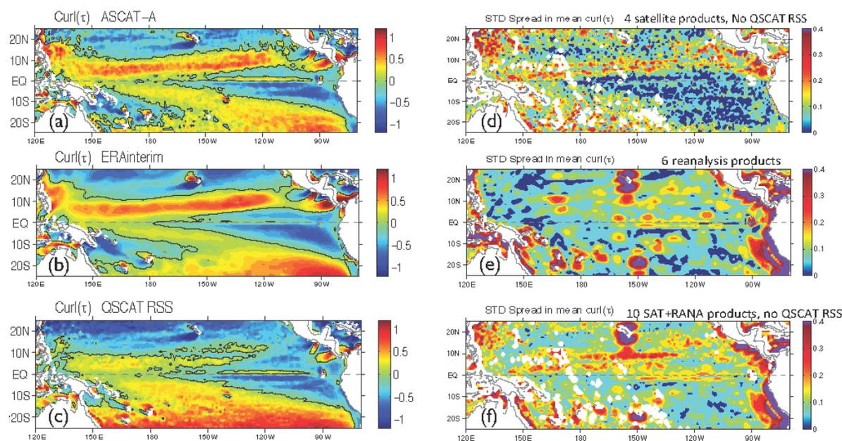
**Figure 3-3: Mean wind stress curl averaged over the two-year ASCAT/QuikSCAT overlapping period 11/2007-10/2009 (a) ASCAT-A; (b) ERA-interim; (c) QuikSCAT RSS (mean pattern altered when rain-flagged wind vector cells are removed); STD mean differences between (d) 6 reanalysis products (CFSR, ERAi, JRA55, MERRA, NCEP1, NCEP2), (e) satellite (ASCAT-A, QSCAT JPL, QSCAT RSS+rain, WindSAT) and (f) satellite and reanalysis products for the same period. Courtesy of Lisan Yu.**
