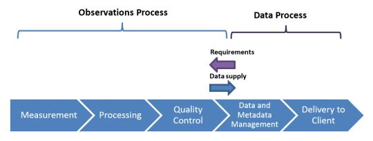
Figure 4.2 - One depiction of the separation of the data process from the observation process (Bureau of Meteorology, personal communication).
