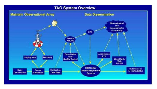
Figure 4.1 – The TAO system, including the data and information system.
